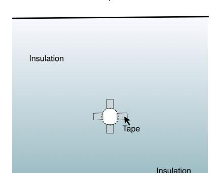
**Helpful Tip:** If you elect to cover the pre-set openings and cut the insulation, cut them before you place the inner liner. Once the openings are cut, tape the insulation to the outer pool. The insulation may move when attaching the inner liner.
