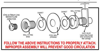
**IMPORTANT NOTE:** When operating your pump and heater, the Gate Valves should be left open. When accessing your cartridge filter for cleaning, they should be blocked. It is a common mistake to start your pump and heater and the Gate Valves are closed. The heater will not turn on in this case.
