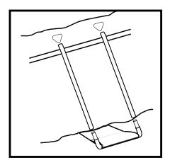
**STEP 9:** When attaching the pool wall insulation, you will need to start about 4 inches from the plumbing openings. So that when you are finished with the insulation, there should be about an 8 inch gap exposing the two plumbing openings.
